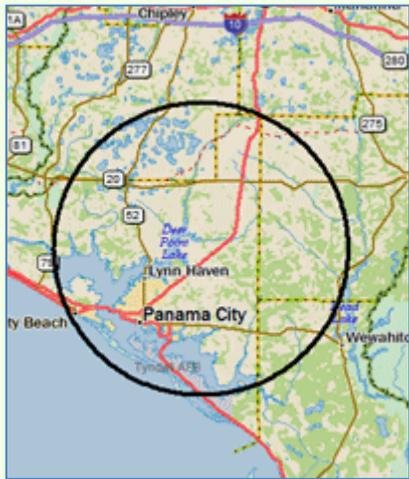
**Example RadioSAFE (RSF.500:10X) signal coverage of up to 20-mile radius (shown above) is possible with an emergency authorization from the FCC. Variables that affect coverage are the authorized power level, terrain, ground conductivity and frequency. Predicted coverage is part of the RadioSAFE engineering documentation package**
