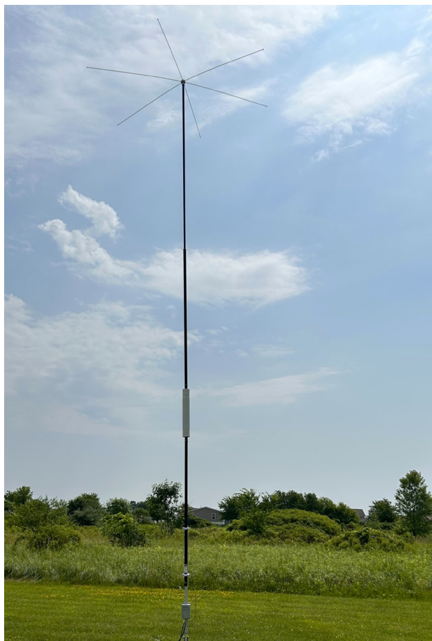
Figure 1 — Paul's 22-foot ground-mounted vertical antenna with combined inductive center loading and capacitive top loading.
